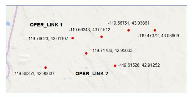
Once the coordinates are plotted as points, the points are converted to lines. The line(s) are built in the same order in which the coordinate pairs are listed in the Excel or text file.
